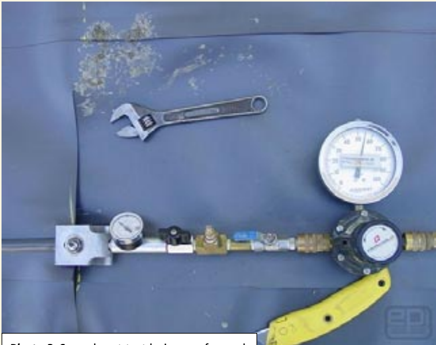
Photo 3. Seam burst test being performed.
